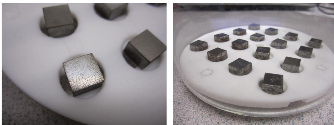
Figure 2-1: (a) Magnified image of carbon steel coupons emplaced in the sample slots of a Teflon holder; (b) image of the Teflon sample holder placed in a modified 2 L beaker.
